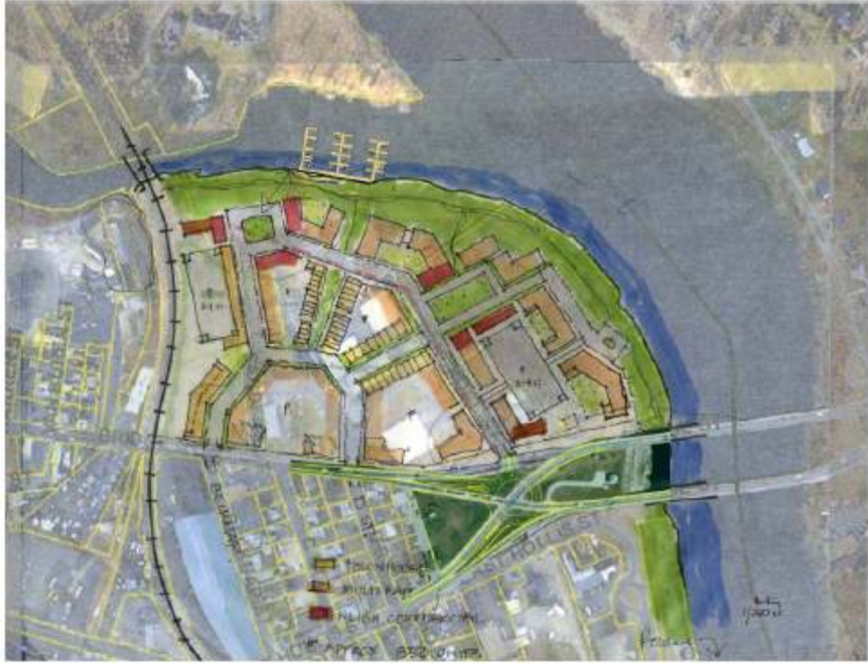
Plan Framework (Alt A): Preliminary study of a roundabout to facilitate access into the site from East Hollis Street, while maintaining bypass lanes to access the bridge.
